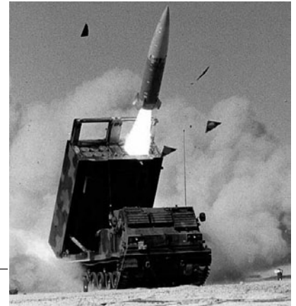
The MLRS systems fires a ATACMS Block 1 rocket composed of 950 sub-munitions (Lockheed Martin)
