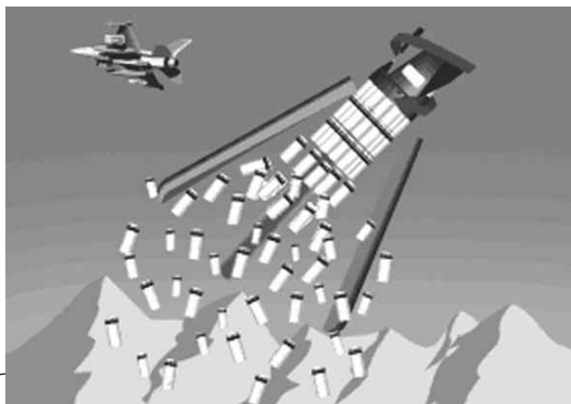
A fighter plane drops a cluster bomb that opens at a designated height and releases more than 100 bombs. (animation BBC)
